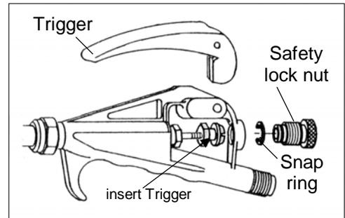
15. Screw the Safety lock nut into the valve body, and then attach the Snap ring.
