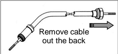
Replace the cable if it is worn or damaged.
