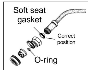
**P.** Hose is leaking at the connection with the tank; leaks when tank is pressurized.
