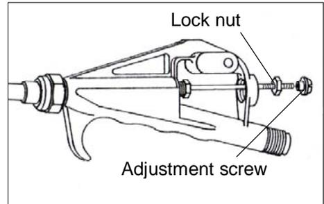
13. Screw onto the cable the Lock nut and the Adjustment screw. Turn the Adjustment screw so the end of the cable is level to the top of the slot in the top of the screw. Tighten the Lock nut against the screw.
