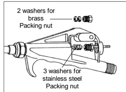
**P.** Extension is leaking at the tip, a constant drip from the tip.
